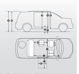
Flexible seating configurations with removable, interchangeable passenger and behind-driver seats. Optionally, the driver seat is removable for a wheelchair driver.
